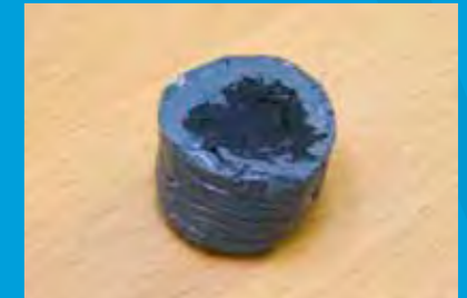
Quick Steel is a two-part epoxy, just knead the product until all colour flecks have gone.
